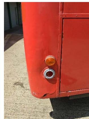
*Rear nearside lower corner – remove filler & reshape corner.*
