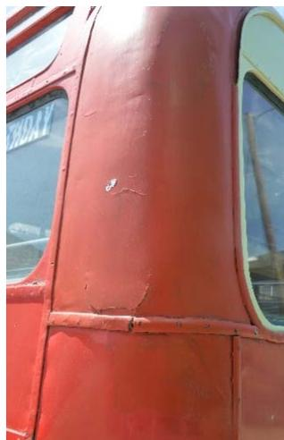
*Rear offside upper corner with body filler separation – remove filler & reshape corner.*
