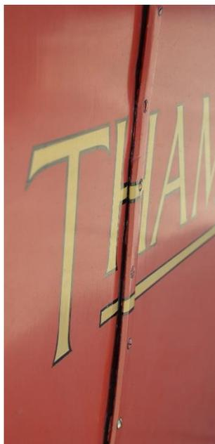
*Offside panel edge cover mouldings separating due to hidden deterioration of timer in body pillar*
