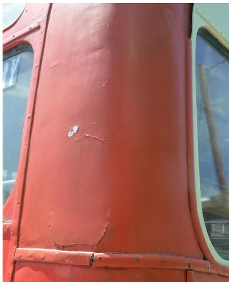
*Rear offside upper corner with body filler separation – remove filler & reshape corner.*
