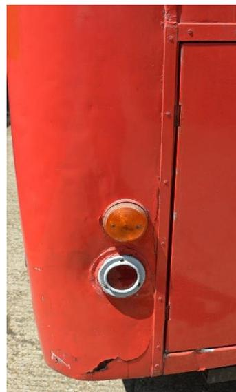
*Rear nearside lower corner – remove filler & reshape corner*
